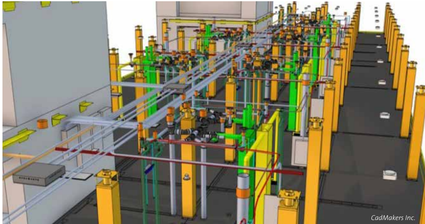
Detailed modelling of the building systems, in coordination with the mass timber structural elements.
