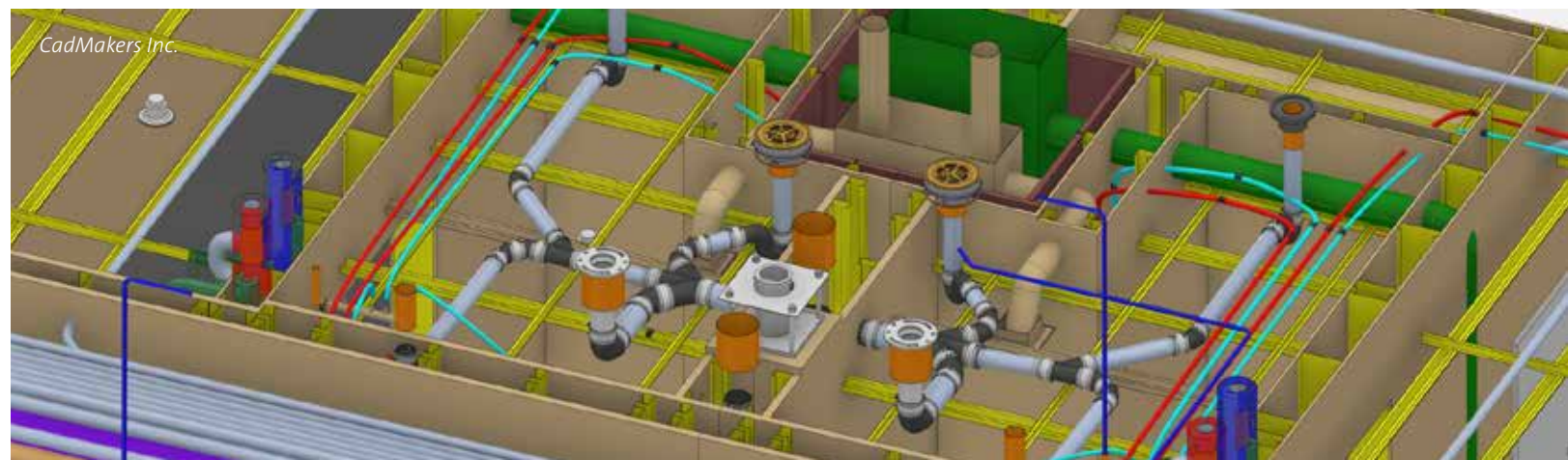
The detailed virtual model allowed the team to identify potential clashes and constructability issues and it helped the team coordinate the layout for pre-fabrication of the CLT panels.
