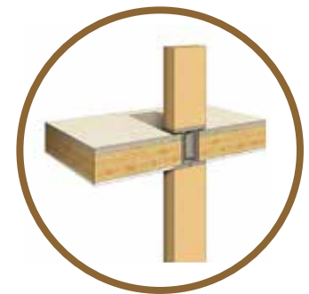
Partial encapsulation of CLT panel, for fire safety during construction
