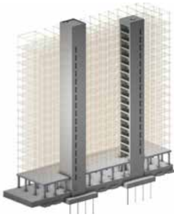
Cast in place reinforced concrete structure Ground-floor columns, transfer slab, and concrete cores
