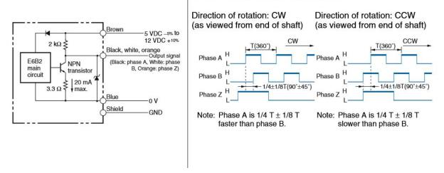
Figure 6.2 - Rotary Encoder Outputs Diagram
