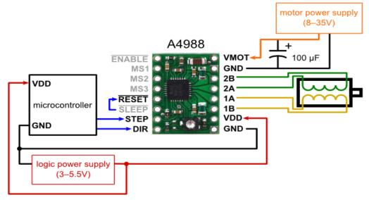
Figure 6.1:Circuit Diagram of the motor driver
