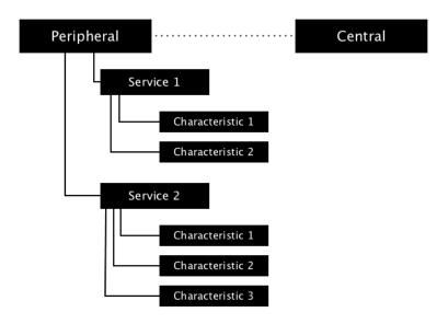
Figure 4.1 Block Diagram of an Example Peripheral & Central
