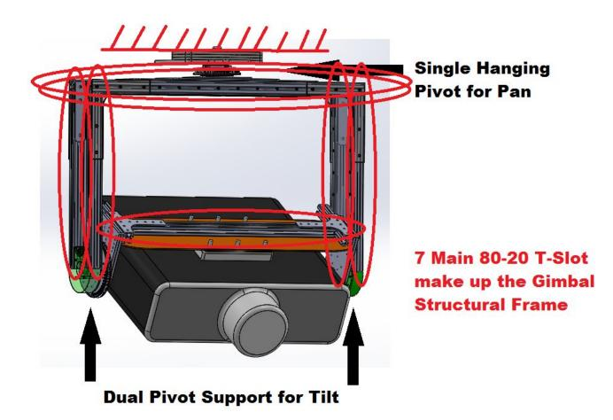
Figure 2.1 - Gimbal Style Structural Frame
