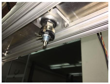
Figure 3.1 Position of potentiometer
