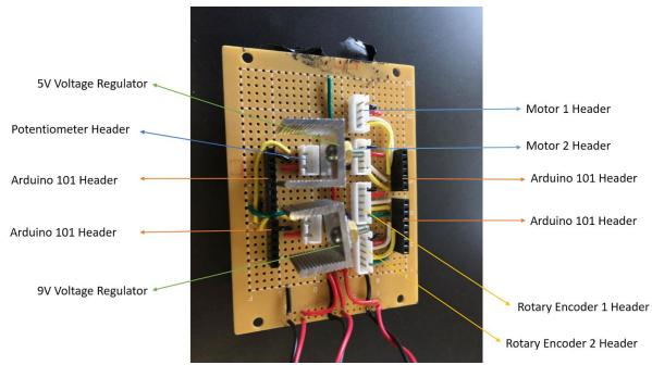
Figure 6.4- Protoboard Circuit Diagram
