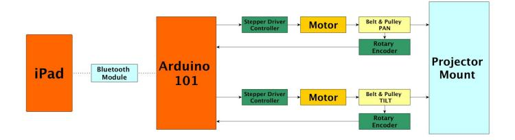
Figure 1.1 - System Block Diagram Project Overview
