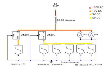
Figure 3.3 - Power Distribution Circuit Diagram
