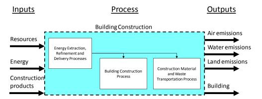
Figure 5 - Generic unit processes considered within Building Construciton by Impact Estimator software.
