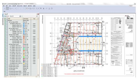
Figure 10 - Autodesk Quantity Takeoff for Beams & Columns
