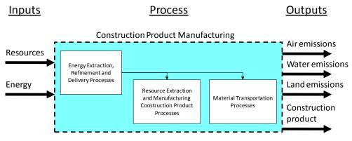
Figure 4 - Generic unit processes considered within Manufacturing Construction materials by Impact Estimator software.
