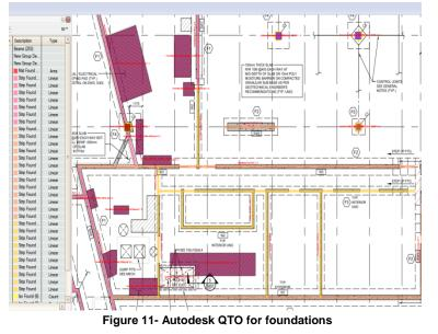
structural drawings (Fast + Epp) S200 & S 201 using Autodesk QTO. Input parameters for Athena IE like concrete strength, fly-ash percentage etc., were taken from structural general notes drawing S100 & S101. Concrete strength for foundations was reduced from 4350 psi to 4000 psi due to the limitation in
