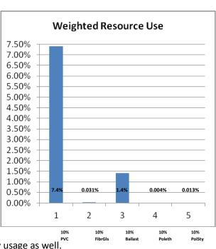
In our study, as evident from the primary energy use "PVC roofing membrane" shows the highest peak of resource usage which in retrospect explain higher energy usage as well.
