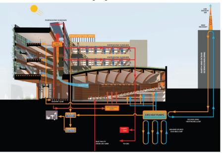
Page 39 of 80 Figure 16 – CIRS Heating system highlighting heat exchange between EOS
