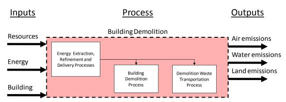
Figure 7 - Generic unit processes considered within Building Demolition process by Impact Estimator software.
