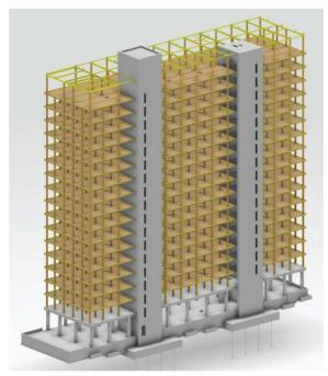
Figure 2: Hybrid structural system (Courtesy Fast + Epp)
