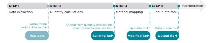
We also identified the different types of BoM created throughout the LCA process as the project data is manipulated into a format that can be assessed using an LCA software tool (see Figure 2):
