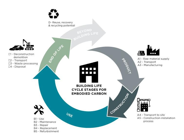
Figure 2: Embodied carbon building life cycle stages and modules per EN 15978:2011<sup>6</sup>
